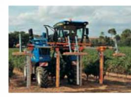
**TRIMMER ST 120 PROVITIS** Adjustable cutting bars with rotary blades of 430mm. rotating at a speed in the range of 2000rpm. The trimmer might be supplied in 2 models (one row or one and two half rows) with cutting heights of 123, 142 and 175cm.
