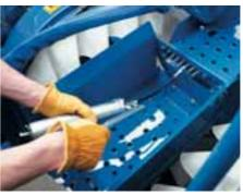
**CENTRALIZED GREASING** To facilitate and reduce maintenance, all harvester head grease points are grouped at a single point. Automatic greasing is available.
