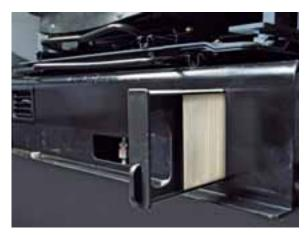
Airconditioning filter, positioned under the seat, can be easily removed without tools and from ground level, for easy cleaning.
