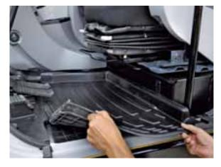
Detachable two-piece floormat with handles for easy removal. A floor drain is located under the mat to facilitate inside cab cleaning.
