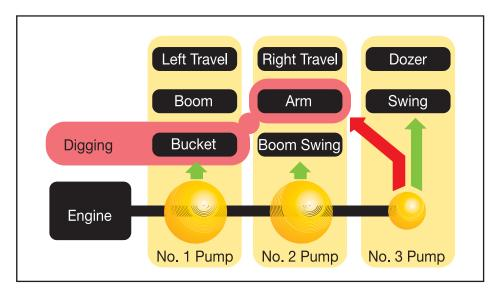
The instant the machine begins to dig, extra output from the third pump (which otherwise powers the swing and dozer circuits) is directed to the arm circuit for added power. This ensures fast and smooth arm operation even under heavy loads.
