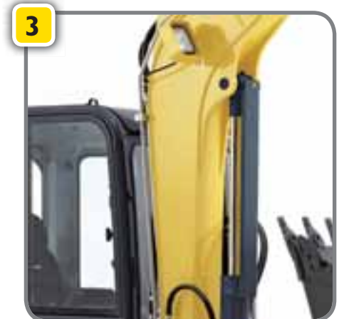
Boom cylinder is protected in every working condition
