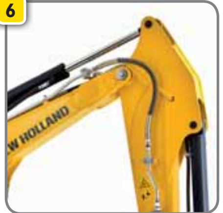
Reinforced boom/arm connection
