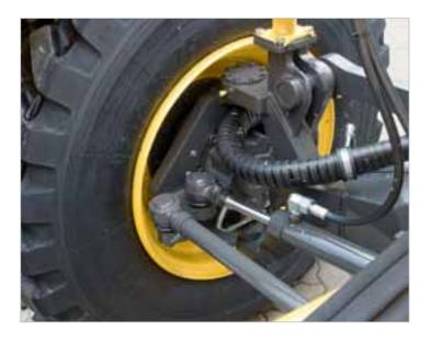
heel lean adjustment permits sound and safe work on embankments with no thrust loss from repeated steering adjustments, and guarantees precision tracking. On the all-wheel drive models, the front wheels are driven by a variable displacement pump and hub-mounted motors. The E.D.C.V. (Electronic Drive Control Volume) uses a hydraulic differential to match oil volume and, hence, the front wheel speed automatically to the speed of the rear wheels.
