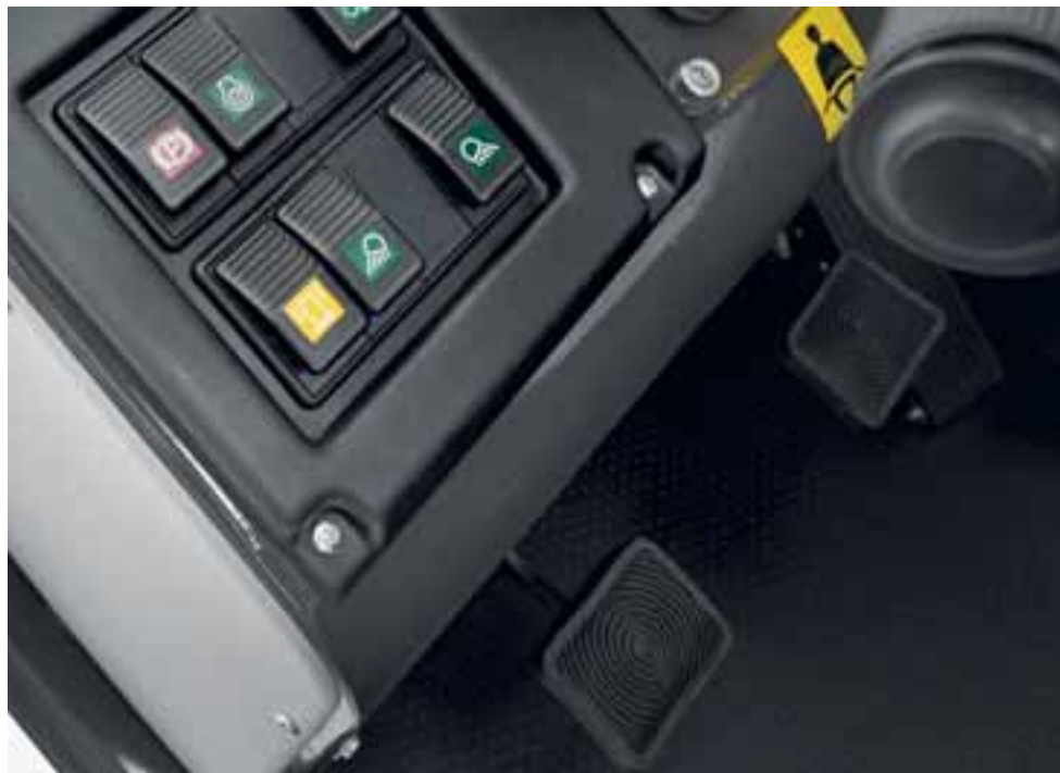
With the inching pedal the driver can modulate the powerful hydrostatic transmission
