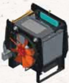
Most wheel loaders mount their radiators back to back. At New Holland we have mounted them to form a cooling module like a box. The benefit is better cooling, in the harshest of environments. In addition, with a programmable reversing fan as standard, cleaning radiators will become a thing of the past.
