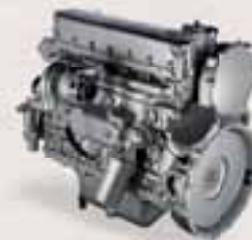
The 9-liter turbo charged engine with intercooler features second generation common rail technology with multiple injections for optimised performance and fuel efficiency.
