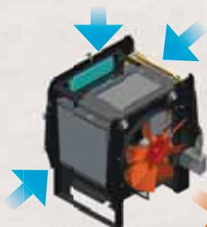
At New Holland we replaced the conventional overlapping radiators with our unique design: we made a box with the radiators. The benefits are longer maintenance intervals and easier cleaning.
