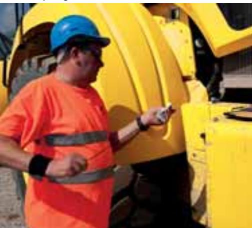
The removal of air filter can be done from ground level in a few seconds
