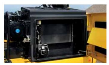
Cooling components (radiator, hydraulic oil cooler and intercooler) are now mounted in parallel, which means increased cooling efficiency for higher component reliability whilst being easier to check and clean.
